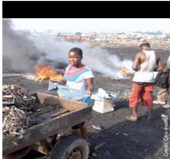
Sorting of cables prior to copper recovery.
